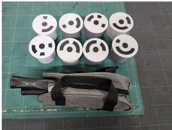
Fig. 2. 3D printed targets and bag containing the stakes and hammer needed for placement.
