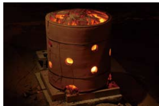
Firing test of the restored kin sumigama.
